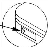
Plug the AC adaptor to the AC adaptor socket on the side. The AC input requirement could be 110,120,220,230 or 240Volts (50/60Hz) depending on the area where used, so please verify that the adaptor is correct
